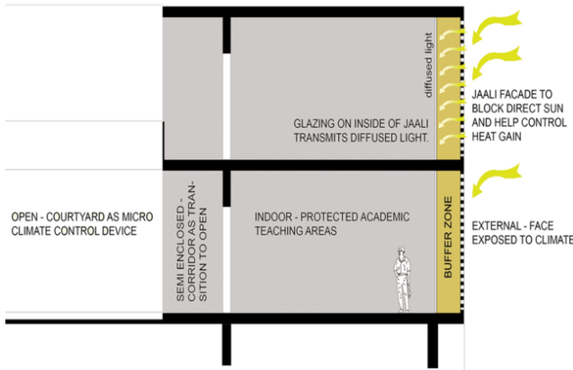
Fig. 22: Double skin by lattice screen
